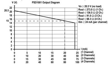
**Short circuit current:** ≥ 24 mA per channel (26 mA typical)
